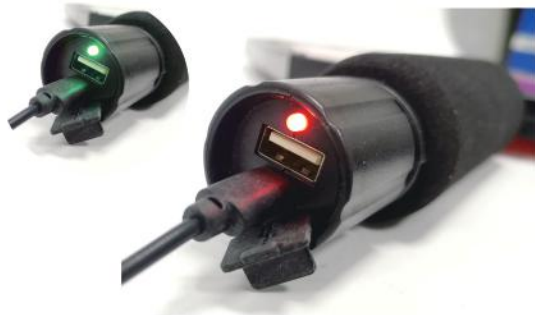
USB terminal for emergency power bank
